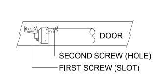
And drill a 3mm hole at this mark. Fasten the **Door Bracket** with one **12mm Screw**. Remove the **Closer** (jamb end first) and drill through the second screw hole. Fit the second **12mm Screw** in the **Door Bracket** and refit the **Closer**.
