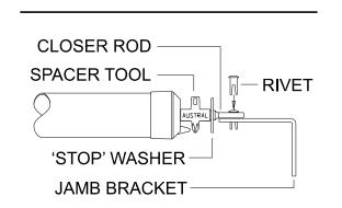
Place the **Stop Washer** over the **Rod** and place the **Rod** onto the **Jamb Bracket**. Slip the forked **Rivet** supplied through both. <u>**Do not**</u> deform the legs of the **Rivet** or remove the **Spacer Tool** at this stage.
