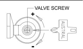
• Open the door, remove the **Spacer Tool** from the **Closer Rod**. Test the **Closer** and adjust the **Valve Screw** with **Spacer Tool** to control the closer speed. Deform the **Rivet** with the back of the **Spacer Tool**.
