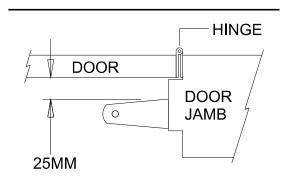
Place the Jamb Bracket on the hinged side of the door jamb, 25mm from the face of the door and 40mm down from the top of the door. Fasten the Jamb Bracket with the three 25mm screws provided.
