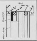
4. For the outside top sash fit the 113 mm stop to jamb at the sill against the inside face of the outer lining (see diagram). Alternative stops may be used provided they stop the sash 113 mm from the sill. Raise bottom sash (inner window) to stops and secure temporarily.
